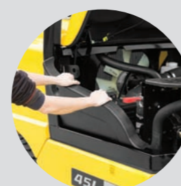
Removable Side Panels for Ease of Service
