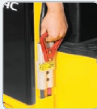
Battery Disconnect Lever
