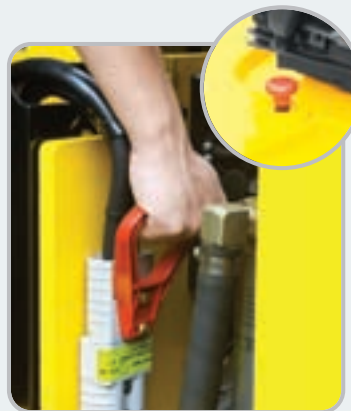
Battery Disconnect Lever
