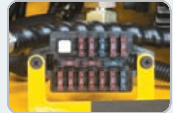
A centralized fuse box for easy inspection
